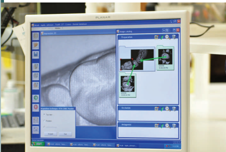
Photographic images are taken of the dies and displayed on the inlab software. The technician defines the margin and adds proper support where needed.
